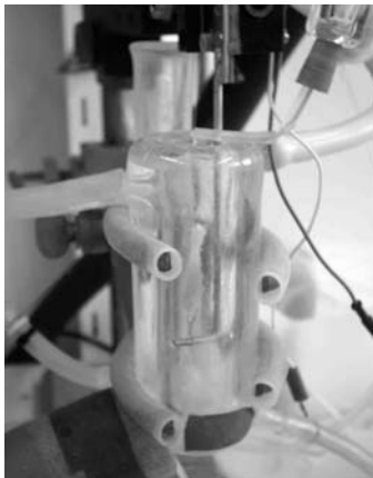
Fig. 7: In vitro contraction test: a piece of fresh porcine lumbar fascia is vertically suspended inside an organ bath. The tissue is isometrically stretched for 1 hour; then a pharmaceutical agonist is added into the bath and any tension changes in the tissue are registered.
